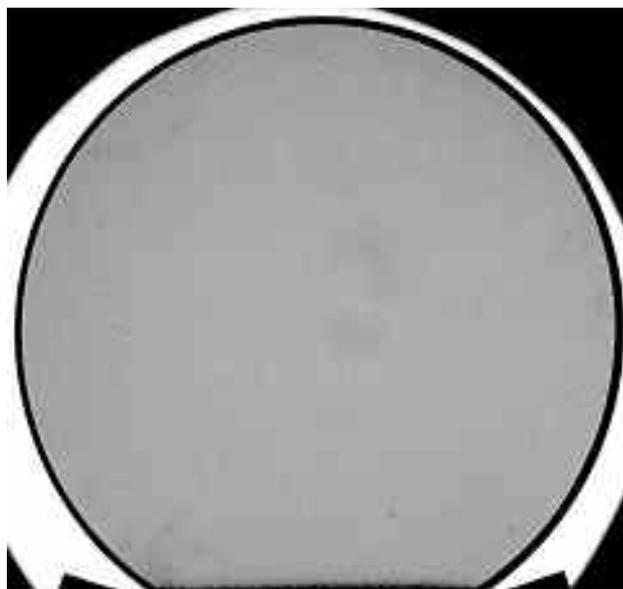
**Figure 6:** Shadowgraph of a specially selected and produced 250 mm diameter ZERODUR<sup>®</sup> blank. No striae above 10 nm wavefront deviation are visible in this setup.
