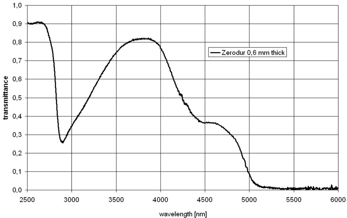
**Figure 3:** Transmittance curve of ZERODUR® at 0.6 mm thickness.
