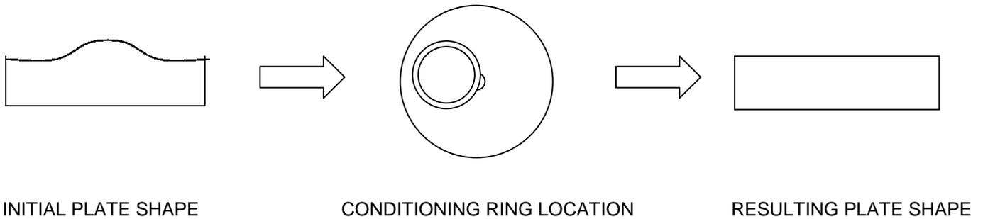
**Figure 6:** Schematic illustration showing a two step conditioning process. The top figure shows a plate with a wavy surface due to a small lapping fixture being used without a conditioning ring. The initial conditioning is completed with the conditioning ring on the outer diameter of the plate. Once the outer portion of the plate has been lapped down, the conditioning ring is moved to the center of the plate to lap it flat.
